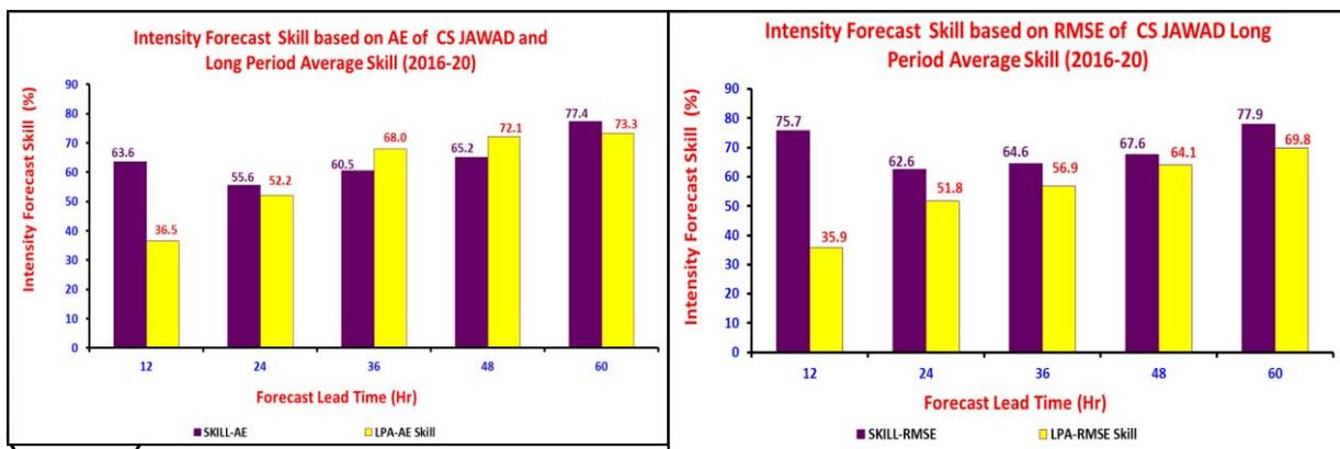
**Fig. 4.3.5.5: Skills based on (a) Absolute errors (AE) and (b) Root Mean Square errors (RMSE) in intensity forecast (winds in knots) of CS “JAWAD” as compared to long period average (2016-20)**
