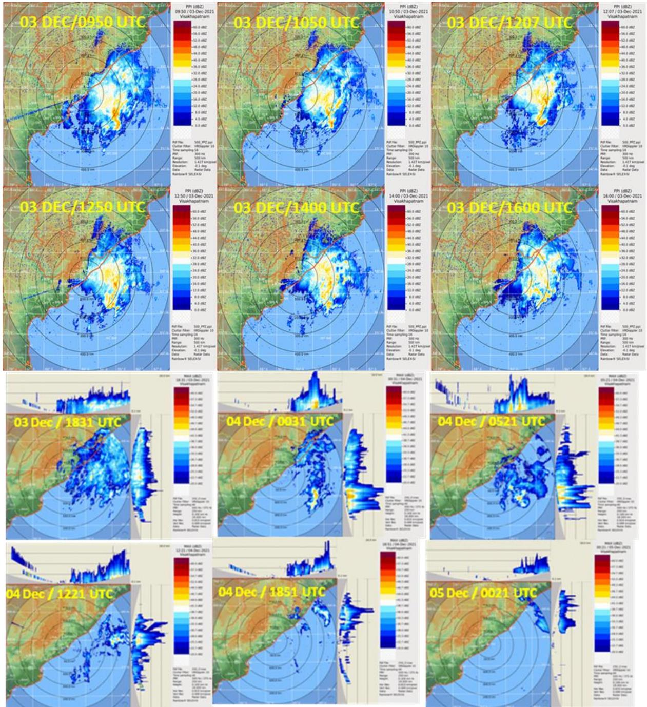
**Fig.2.11.6(a): Maximum reflectivity (dBz) imageries from DWR Visakhapatnam during 03 Dec-06 Dec, 2021 in association with CS Jawad**
