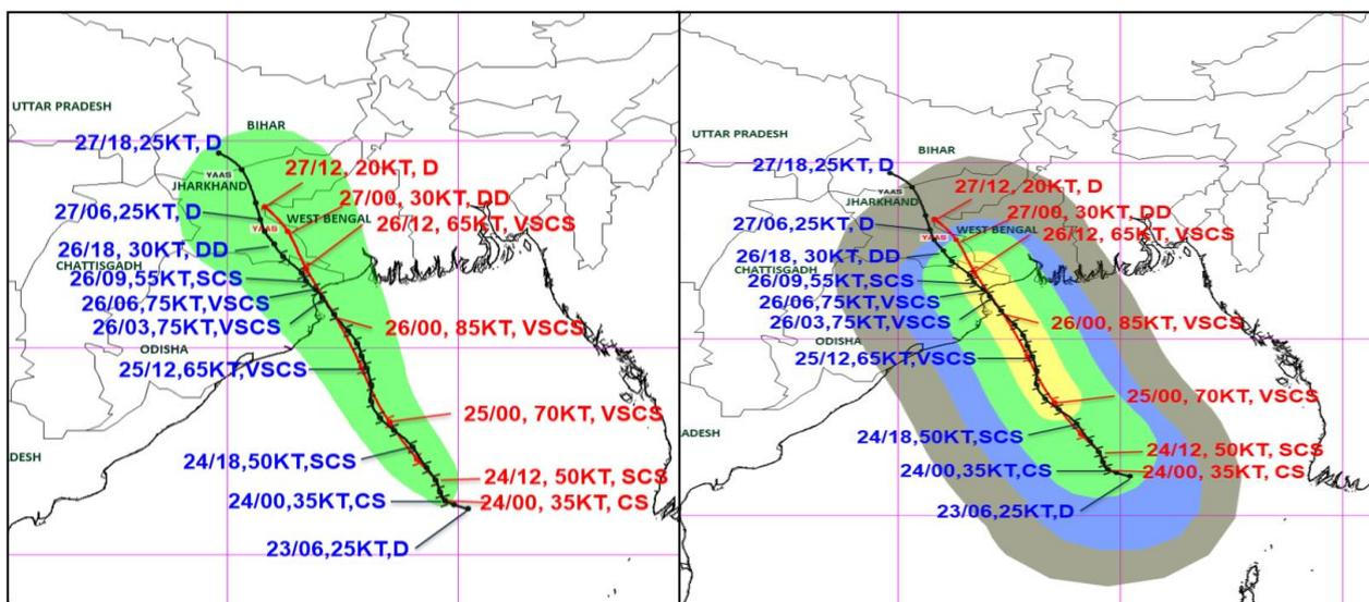
Fig.4.3.2.2: Observed track (23-28 May) and forecast track issued at 0830 IST based on 0530 IST observations of 24<sup>th</sup> May (about 54 hours prior to landfall) demonstrating accuracy in track, intensity and landfall
