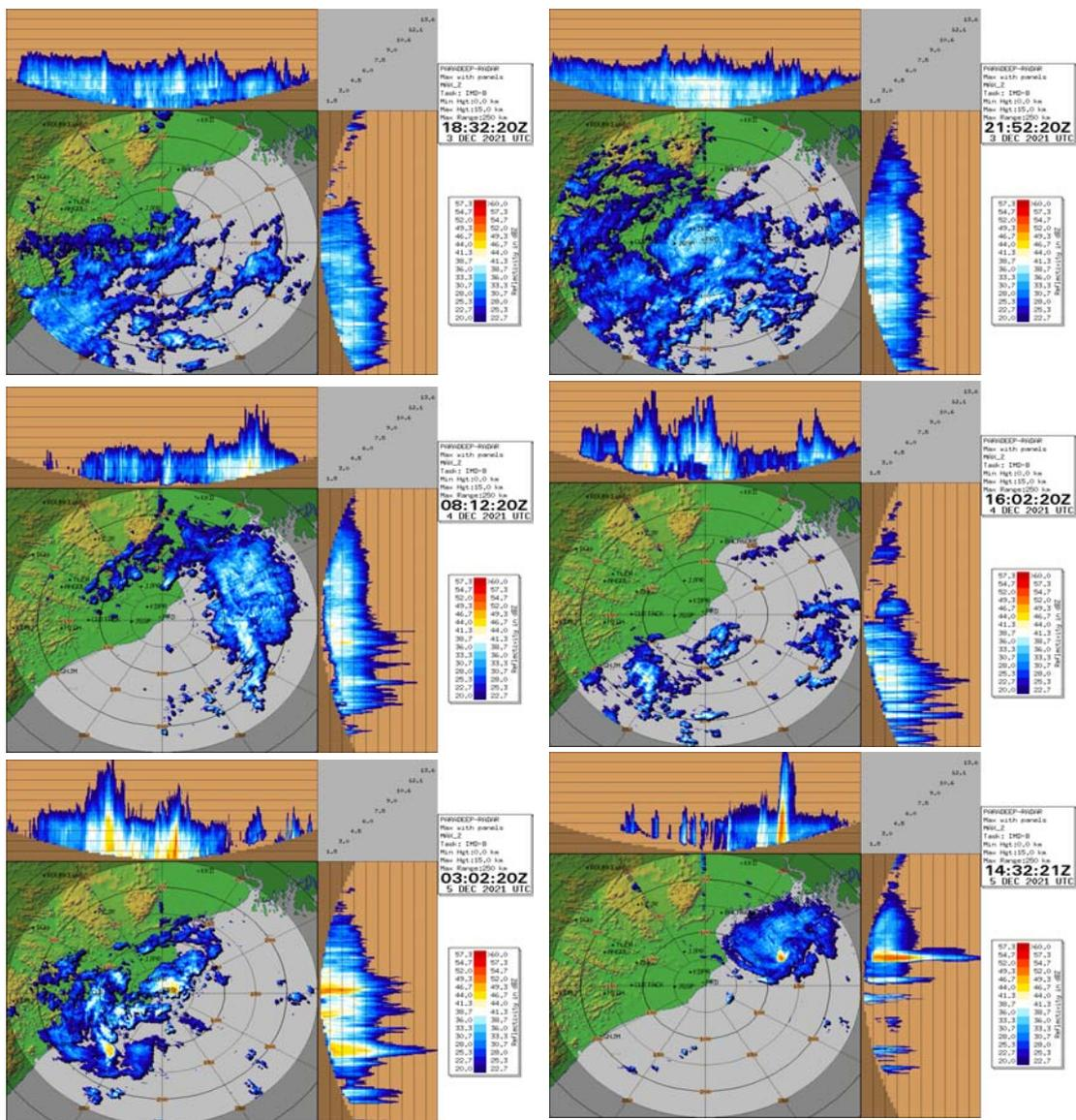
**Fig.2.11.6(d): Maximum reflectivity (Z) imageries from DWR Paradeep during 03 Dec-05 Dec, 2021 in association with CS Jawad**
